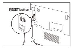
3. Press the TEST button lightly with a sharp edge such as a pen tip. The depressed RESET button will stick out again. This is the end of the check procedure.
